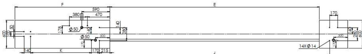
1. Install the ground fixations of the guiding and end post according to the positions indicated on the foundation plan. Therefore following fixation material is required: Chemical anchors M12x160 (minimum 80mm above Finished Ground Level. For anchor depth check installation manual of supplier chemical resin).
